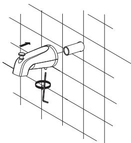
**7** Slip on installation over 1/2" copper pipe: Slide the spout over the pipe with the spout tight to the wall, tighten the set screw to the pipe.
